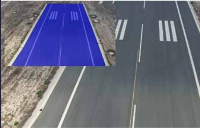
Inspection ► Maintenance ► Infrastructure ► Airport runway Pavement Condition Index inspection - Canard Drone, Spain
