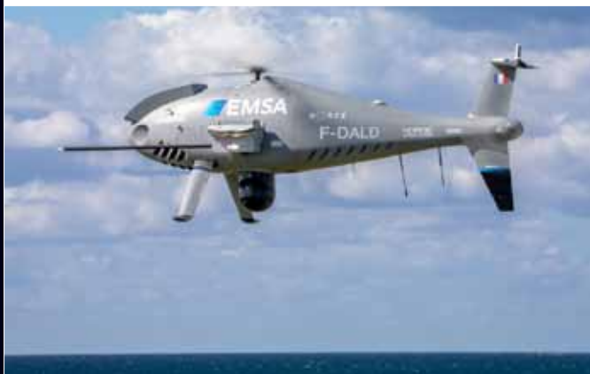
Monitoring ► Environmental Protection & Conservation ► Pollution (aerial, maritime, terrestrial) Camcopter S-100 monitoring ship sulphur emissions for EMSA - Schiebel, Austria
