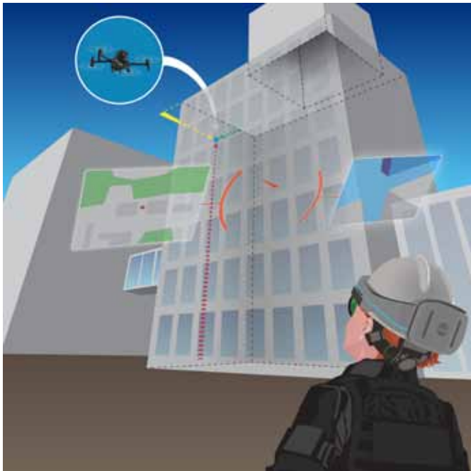
Fig. 2 - AirHUD enables the pilot to even fly the drone behind obstacles and still see their location and intuitively their relationship to their surroundings.
