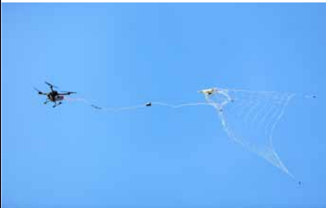
Special Purpose ▶ Security & Law Enforcement ▶ Interception of hostile/illicit drone DroneCatcher - Delft Dynamics, The Netherlands
