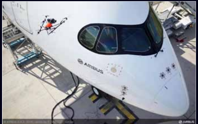
Inspection ► Maintenance ► Aircraft hull exterior inspection Airbus A350 hull inspection (Aircam Project) - BizLab Toulouse, France (Airbus)
