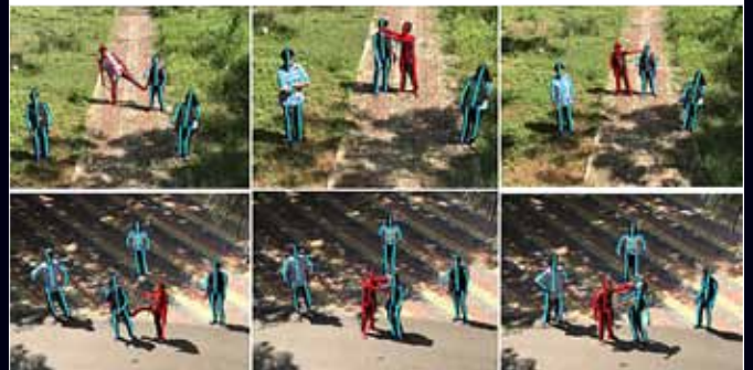
Identification ▶ Security & Law Enforcement ▶ Suspected criminals/pillagers/rioters The Drone Surveillance System highlights violent individuals in red and neutral individuals in cyan University of Cambridge, UK & National Institute of Technology, India - Indian Institute of Science, India & IEEE, USA
