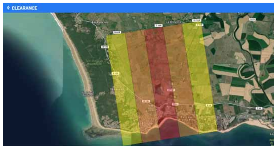
Fig.1 - Red strip requires authorization for every flight. Orange: authorization is needed above 50 m. Yellow: above 100 m. The flight altitude limits have to be computed using Aerodrome Reference Point altitude, not altitude of terrain below the drone.
