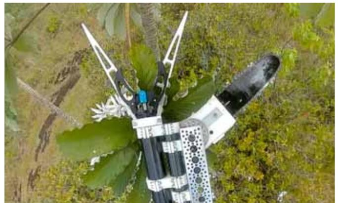
Drone Fitted with Chainsaw (tree pruning)
