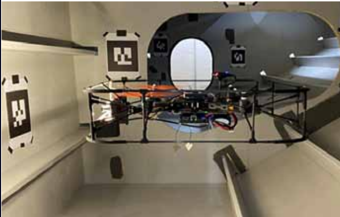
Inspection ► Maintenance ► Shipping ► Ship ballast tank Drones for safety inspection of ships pass test - Technical University of Denmark
