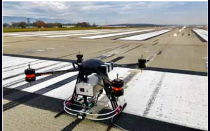
Measuring ► Maintenance ► Instrument Landing System measurements OnyxStar ATLAS - Altigator, Belgium
