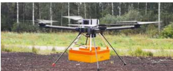
Lava Flow Mapping - General Directorate of Safety and Emergencies of the Canary Islands Image: Copernicus Emergency Management Service Tundra drone with Ground Penetrating Radar Hexadrone, France
