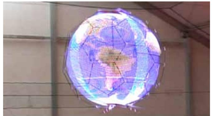
Spherical Drone with Projection on Exterior (indoor flight)
