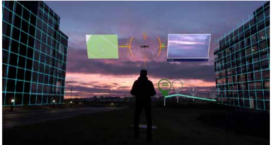
Fig. 1 - The augmented reality view given to the drone pilot with AirHUD, showing the drone indicator always pinpointing drone's location, with map and video feeds beside it, and also mission waypoints in real world locations, and even building meshes that enable real-time distance indication between the drone and the nearest building.
