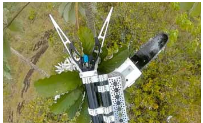
Drone Fitted with Chainsaw (tree pruning) University of Hawai'i, USA
