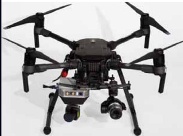
Drone for aircraft fuselage inspection
