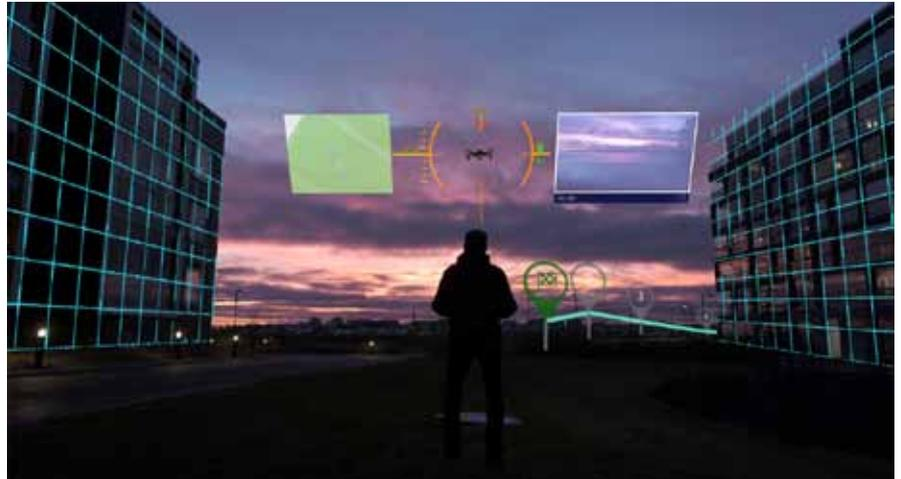
Fig. 1 - The augmented reality view given to the drone pilot with AirHUD, showing the drone indicator always pinpointing drone's location, with map and video feeds beside it, and also mission waypoints in real world locations, and even building meshes that enable real-time distance indication between the drone and the nearest building.
