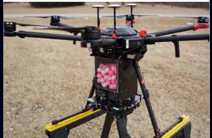
Fireball Hopper (to create controlled burns) to contain forest fires ▶ Forestry & ▶ Public Services & Safety Ignis by Drone Amplified, USA
